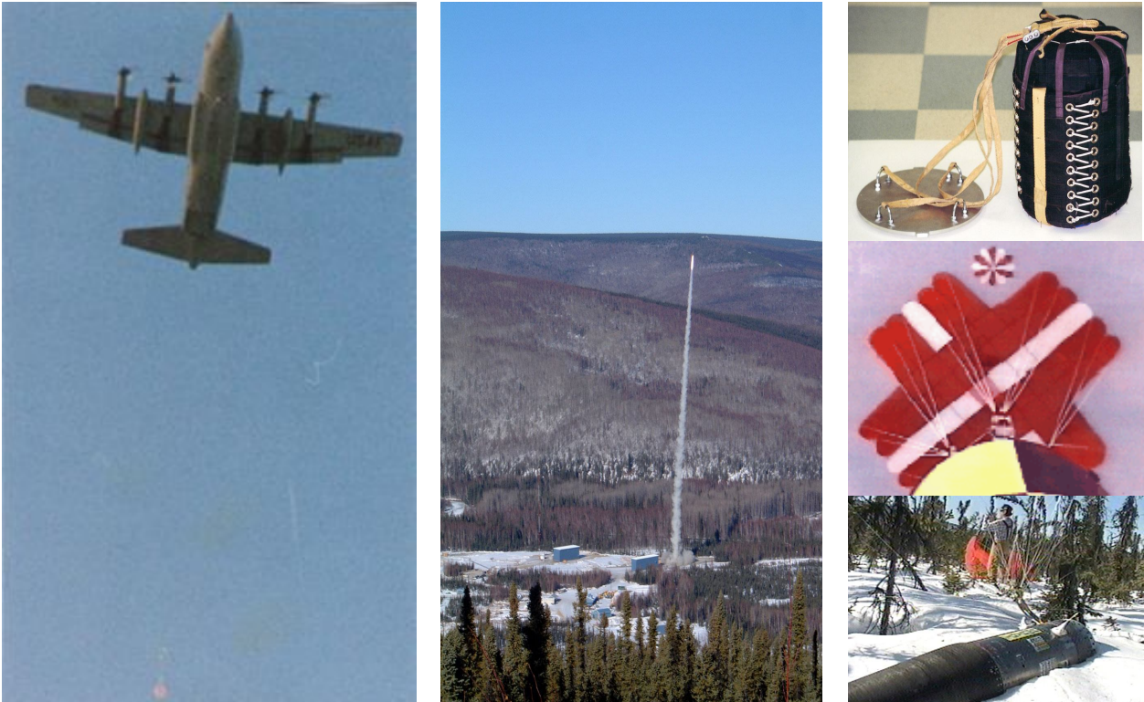
Figure 1: (LEFT) - Parachute system flight qualified by drop testing from C-130 aircraft. (MIDDLE) - Parachute system successfully flown to space and back on NASA/Orion rocket launched from Poker Flats, Research Range, Alaska. (RIGHT) - Top: Packed parachute system, Middle: Fully deployed parachute recovery system, Bottom: Recovered Rocket payload.
