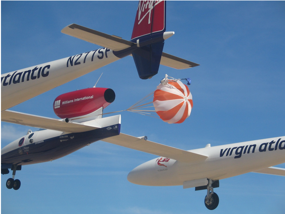
Figure 1: Deployed left drag chute on first test flight March 5, 2004. Note mirror above cockpit for pilot to confirm drag chute deployment.
