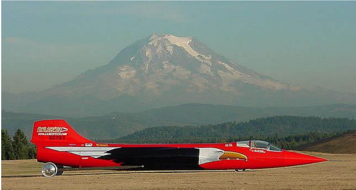
Figure 1: Full side view of the North American Eagle F-104 jet car with high speed aluminum wheels on display with Mount Rainer in the background in Washington State which is the home of this project.
