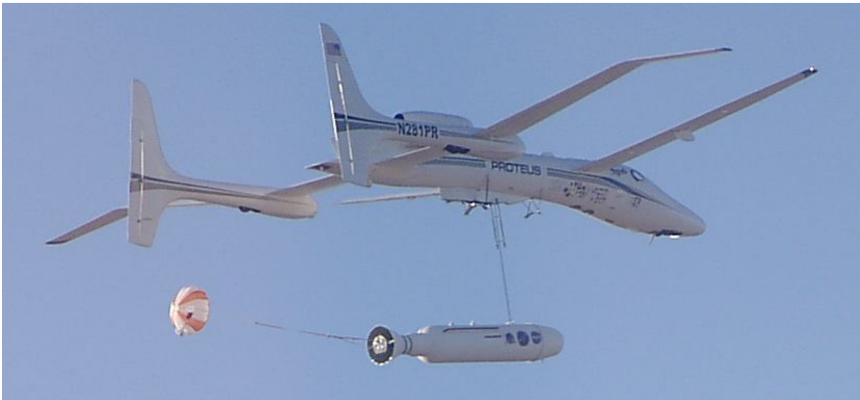
Figure 1: Rocket booster drop test from Scaled Composites Proteus jet with guide surface orientation parachute deployed.
