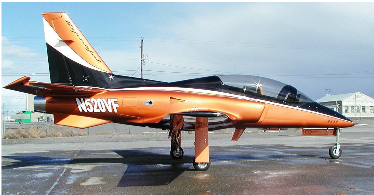
Figure 1: Viper Aircraft all carbon fiber experimental Mark II Viper Jet with performance unmatched by any other very light jet. Photo: Used with permission of Viper Aircraft Corporation.
